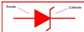
Zener diode is used in voltage regulator.
