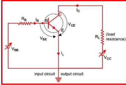
In the above diagram CE circuit is shown using an n-p-n transistor. In this case,
