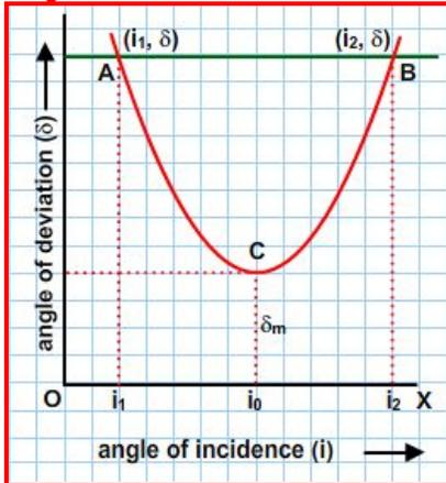
So, for every prism there is a fixed angle of incidence for which the deviation suffered by a ray of light traversing the prism becomes minimum. This minimum angle is called the angle of minimum deviation of a prism. The position of the prism in which the value of the deviation becomes minimum is called the position of minimum deviation of the prism. This position of the prism is unique, i.e., for only one position of the particular prism, the deviation becomes minimum.
